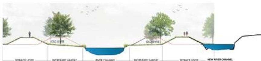
Cross section, river setback levee, Missouri River, US
