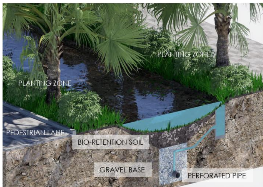
Bioswale typical section. Source: Citilinks
