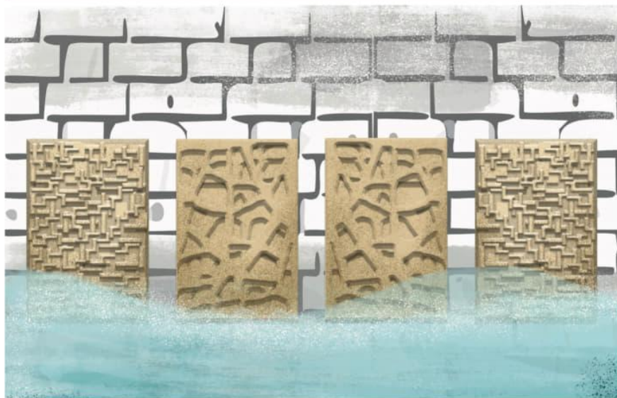
Eco-engineered Tiles Enhance Marine Biodiversity on Seawalls, Hong Kong. Source: ADB
