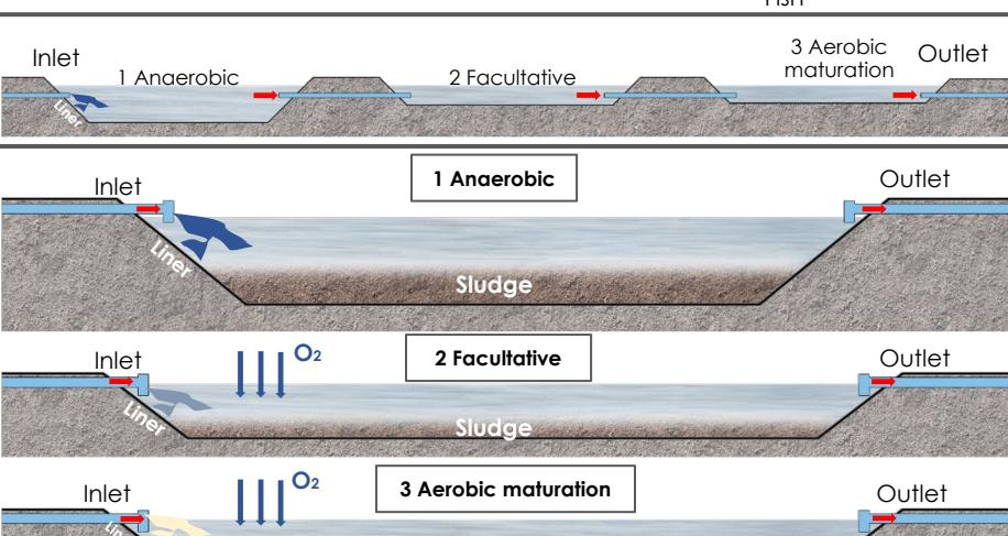
**Wastewater Stabilization Ponds (WSPs)** function individually or in series, with three types: anaerobic, facultative, and aerobic (maturation), each with specific roles. WSPs are low-cost with high BOD and pathogen removal but require large areas and expert design. The nutrient-rich effluent (e.g., nitrogen and phosphorus) is suitable for agricultural reuse but not for direct discharge into surface waters.
