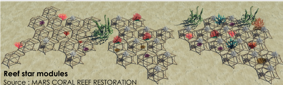
Artificial reef designs : Reef star module and 3D printing tiles structures for coral nurseries.
